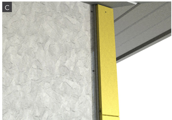
Double Flange Sealant Backer flanking stacked Corners
